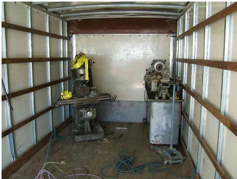
Illustration 5: Rigged mill and lathe, the anchors for the come-a-long was a retired climbing rope belayed off the sides of the truck.
