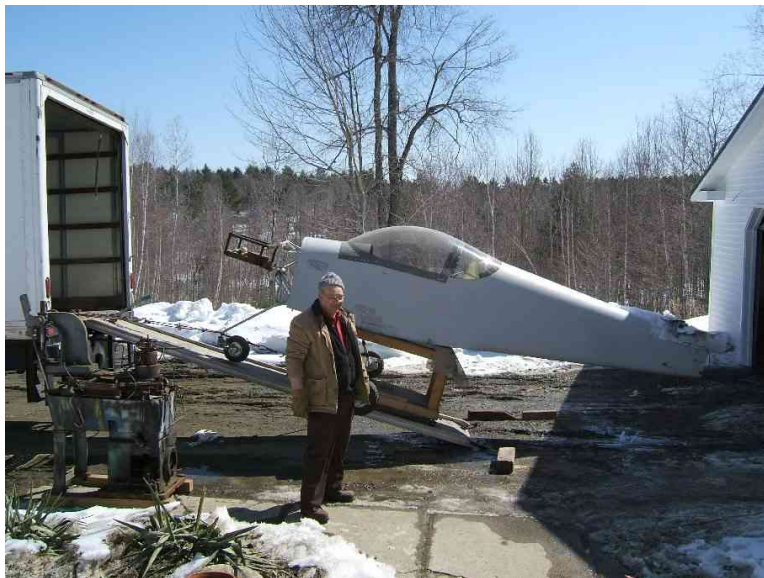
Illustration 7: Note the coupling of the tackle between the nosegear and the work bench
